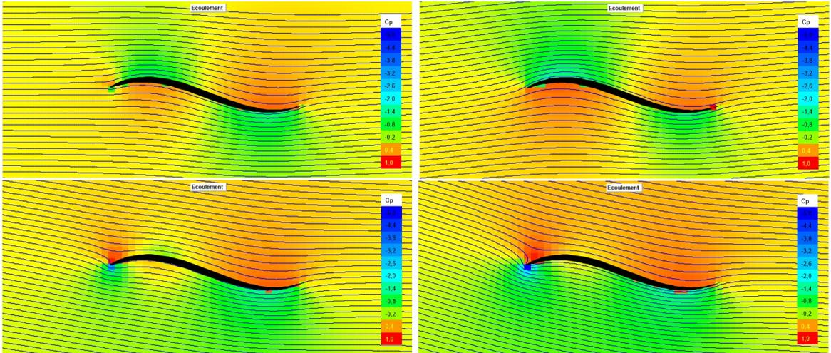
Figure 4: Flow maps for angle of incidence ( $0^\circ$  top left,  $4^\circ$  top right,  $-6^\circ$  bottom left,  $-10^\circ$  bottom right)
