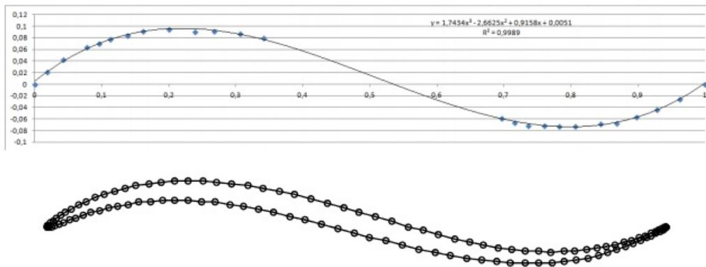
Figure 2: Upper: airfoil used for the theoretical calculation / Lower: airfoil used in the simulation on JavaFoil®
