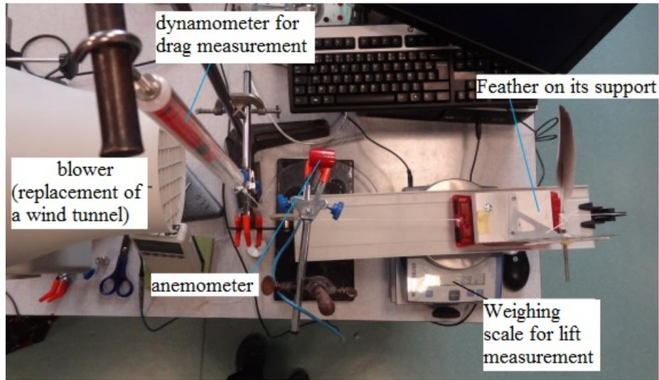
Figure 1: Experimental set-up
