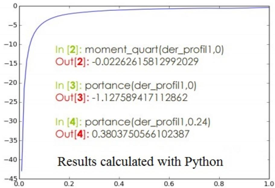
Figure 5: Density of vorticity and calculation of pitching moment and lift associated with the modelled airfoil of RP9
