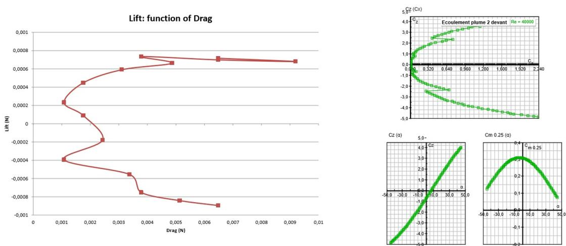
Figure 3: On the left: lift function of drag / On the right: at the top: Lift function of drag, at the bottom left: lift function of angle of incidence and at the bottom right: pitching moment function of angle of incidence
