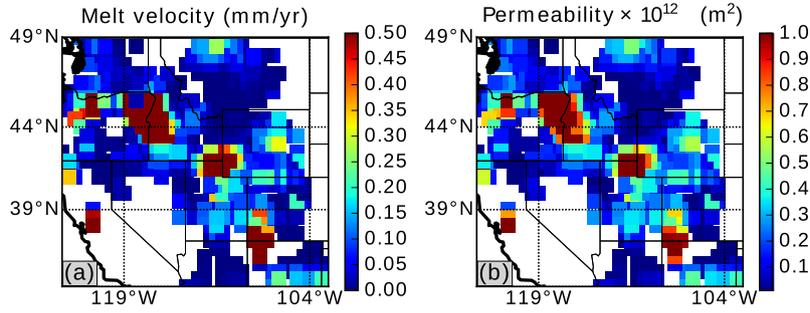
**Fig. 9.** Results from the melt migration calculation. (a) A map of melt percolation velocity at each site. The velocity at each site represents the maximum velocity in a column described by equation (8). (b) A map of permeability at each point calculated using the melt fraction determined from the P-S receiver function analysis.
