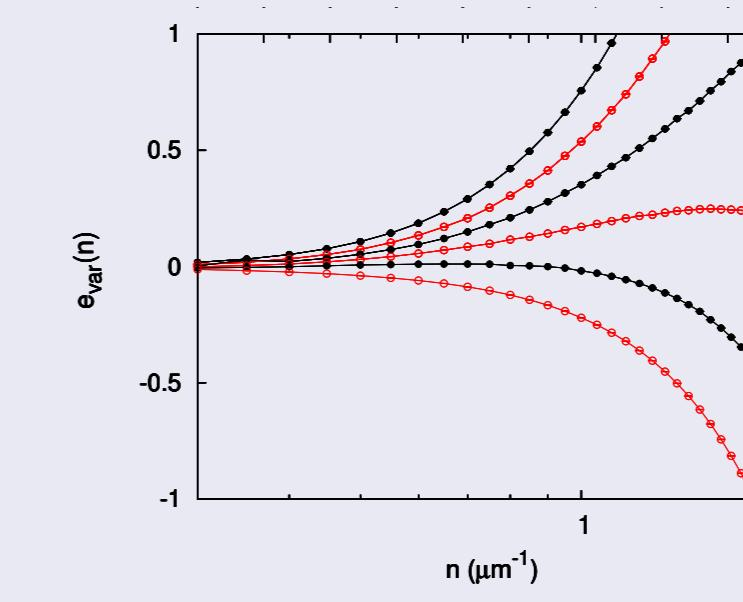
Energy per unit length as a function of atom density for selected scattering lengths. Top to bottom  $a_{1D}/a_0 = 5000, 6000, 7000, 8000, 9000$  and  $10000$
