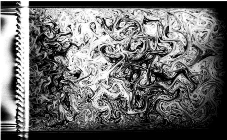
Fig. 1. Grid turbulence in a soap film (from M. Rutgers, 1996 ( http://www.physics.ohio-state.edu/~maarten ). The fluid is moving from left to right, at velocity 2 m/s, across the comb with mesh 0.3 cm, while the total width is 4 cm. Visualization is provided by interference fringes due to small fluctuations of the film thickness (this is like the color patterns in usual soap bubbles). The increase of turbulent scale with distance to the grid is clearly visible, and it has been measured by laser Doppler velocimetry [71] . Note that this technique for producing 2D turbulence has been first developed by Couder [30]
