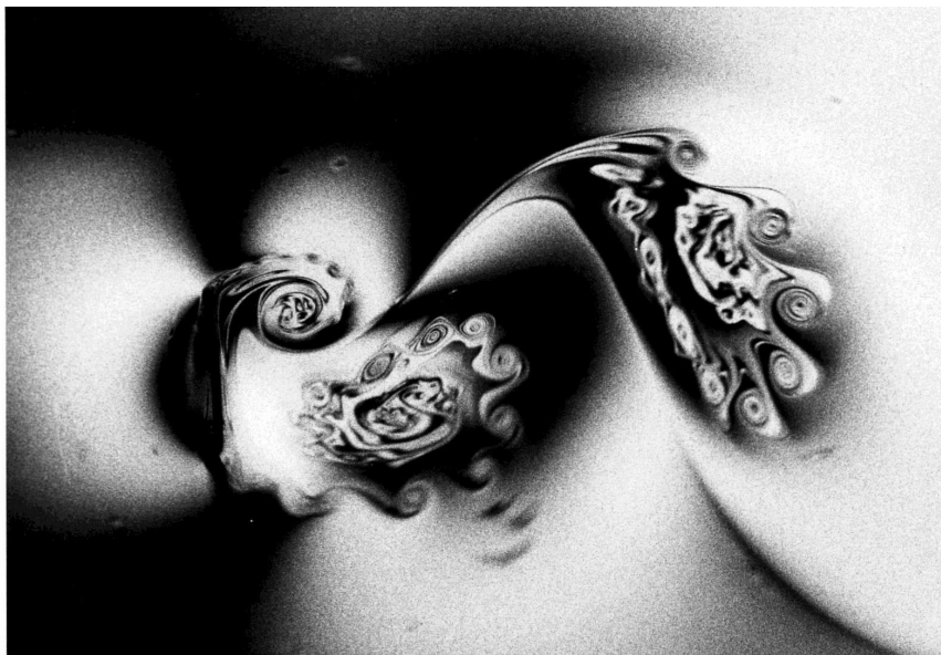
Fig. 17. Wake behind a knife blade in a soap film, the flow comes from the left, (from M. Rutgers, 1996 ( http://www.physics.ohio-state.edu/~maarten )).
