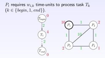
Edge  $e_{k,l}: T_k \to T_l$  in  $G_A$  is labeled with  $data_{k,l}$ : data volume generated by  $T_k$  and used by  $T_l$ Transfer time of a file  $e_{k,l}$  from  $P_i$  to  $P_j$ :  $data_{k,l} \times c_{i,j}$
