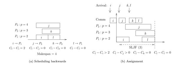
Figure 4: Detailing the last two phases of the SLJF algorithm.
