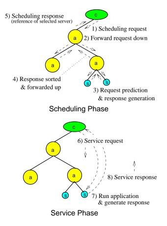
Figure 1: Platform deployment architecture and execution phases.
