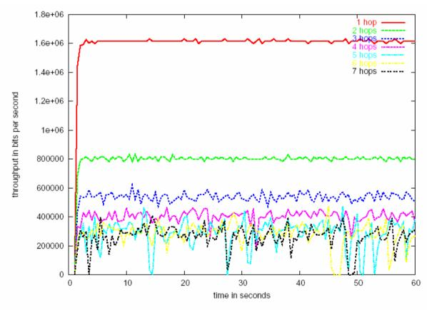
NS2 2 Mb/s 1000 bytes Unicast packets AODV
