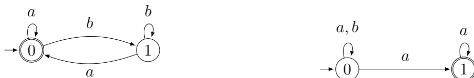
Figure 5: Two Büchi automata. On the left a deterministic one that accepts the infinite words with infinitely many a 's. On the right a non-deterministic one that accepts the infinite words with finitely many b 's.
