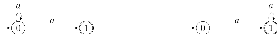
Figure 6: Two automata that are equivalent on finite inputs but not on infinite ones.
