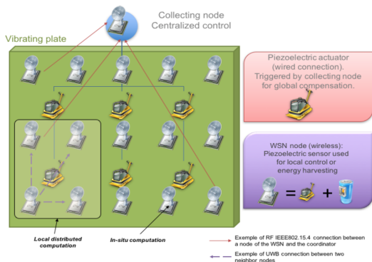
Figure 3: Ampere's vibrating rig [Zieliński 2015]
