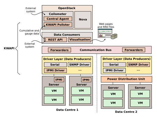
Fig. 2. Overview of KWAPI's architecture.
