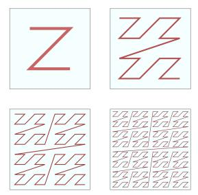
NB: previous analysis need tall-cache assumption  $(M \ge B^2)$ ! If not, use recursive layout, e.g. bit-interleaved layout:
