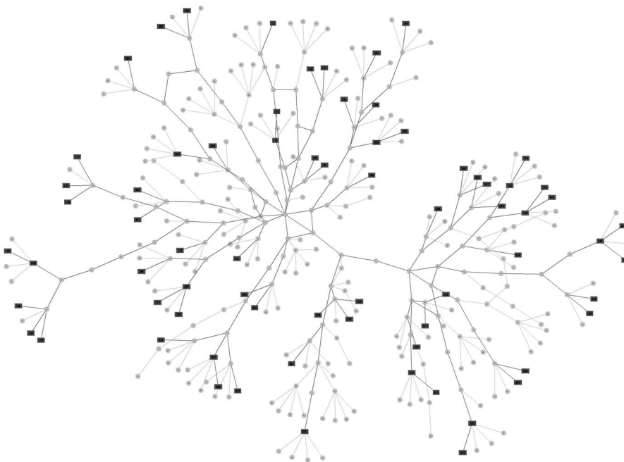
Fig. 4. Second platform. Boxed nodes are selected machine nodes. There are 90 selected machine nodes, connected through 43 routers and 136 communication links.
