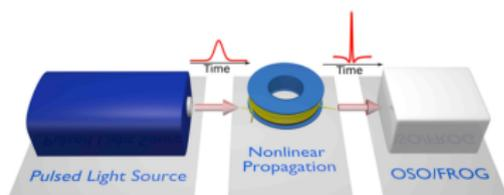
FIG. 3. Schematic experimental setups. The pulsed light source is either a fiber picosecond laser or a spectrally filtered femto-second OPO. The nonlinear propagation of pulses is achieved in a HNLF or in a standard PMF fiber.
