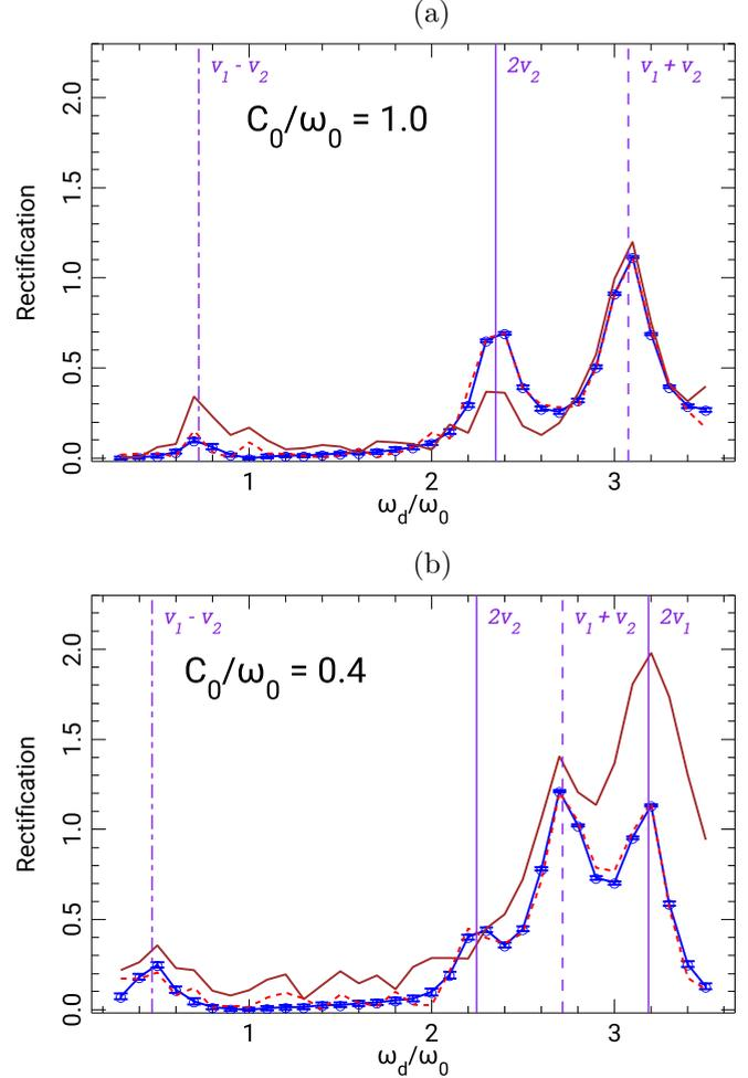
FIG. 2. Rectification coefficients versus the modulation frequency  $\omega_d$  for two values of the coupling constant  $C_0$ : (a)  $C_0/\omega_0 = 1.0$  and (b)  $C_0/\omega_0 = 0.4$ . Brown full line,  $R_Q$ ; blue full line with error bars,  $R_J$ ; red dashed line,  $R_Q$ . The vertical lines show some of the combination of the eigenfrequencies  $\nu_1/\omega_0$ ,  $\nu_2/\omega_0$  of the system of two oscillators.
