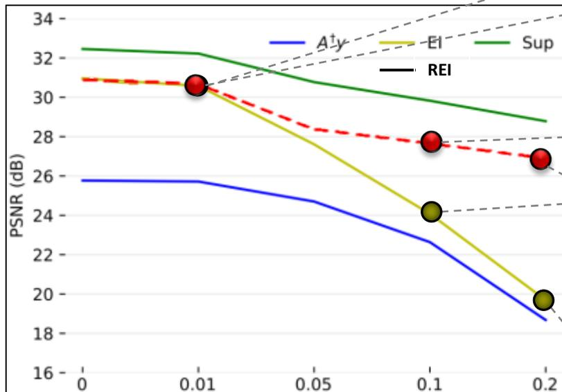
$\sigma$ : Gaussian noise standard deviation  $y \sim \mathcal{N}(u, \sigma^2 I)$  with  $u = \mathbf{A}(x)$ .
