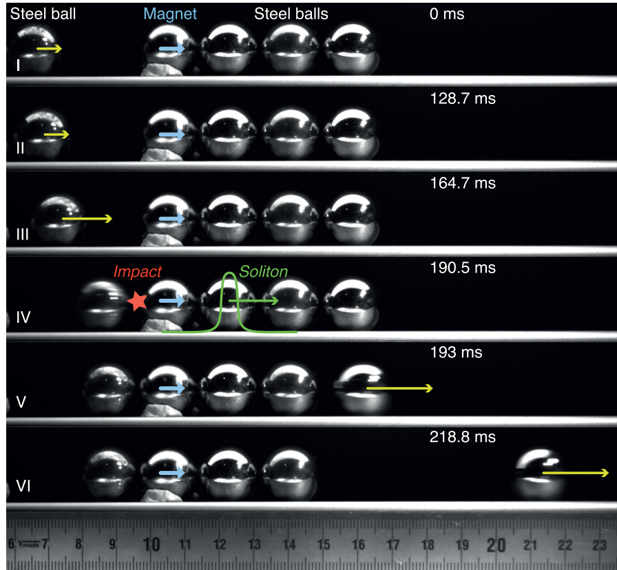
Fig. 1. (Color online) Time sequence (from top to bottom) showing the different phases of the magnetic cannon. A chain of three steel balls initially stuck to the right of a strong permanent magnet (loosely fixed on a rail with putty) is impacted by a steel ball coming from the left and accelerated in the magnetic field of the magnet. Momentum is transferred through the chain and the last ball on the right is ejected with a high velocity. The images are from a high-speed video (resolution: 2048 \times 360 ) acquired at 400 frames per second (enhanced online) [URL: http://dx.doi.org/10.1119/1.4979653.1 ].
