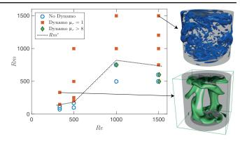
FIG. 1. (Re, Rm) parameter space showing nondynamo (blue empty circle) and dynamo runs (red square) and the dynamo onset (black dotted line) for  $\mu_r = 1$ . Below the dynamo onset at  $\mu_r = 1$ , dynamos were observed for  $\mu_r > 8$  (green diamonds). Right: Isocontours of the time-averaged dynamo magnetic energy field in the growing phase for Re = 333 and Re = 1500 (*Pm* = 1).
