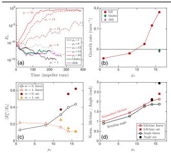
FIG. 2. (a) Time evolution of magnetic energy  $E_b$ , (b) dynamo growth rates, (c) dynamo energy ratio in modes m = 0 and m = 1, and (d) normalized lifetime of the magnetic field line winding number in the vicinity of the impellers and as a function of  $\mu_r$ . See the text for details.
