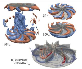
FIG. 4. (a)  $H_z$ , (b)  $H_r$ , (c)  $H_{\phi}$  isoamplitude contours (red, positive value; blue, opposite negative value), and (d) magnetic streamlines colored by the  $H_{\phi}$  value. Re = 1500, Rm = 500, and  $\mu_r = 14$ .
