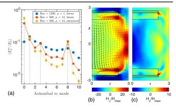
FIG. 3. (a) Azimuthal mode decomposition of magnetic energy, (b) azimuthally averaged  $H_{\phi}$ , and (c)  $H_z$  components normalized to the maximum value in the linear regime for Re = 1500, Rm = 500, and  $\mu_r = 14$ . (b) Vectors show the poloidal dynamo field.
