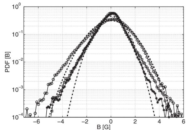
FIG. 6. PDF of the fluctuations of the induced magnetic field:  $B_x$  ( $\circ$ ),  $B_y$  ( $\square$ ),  $B_z$  ( $*$ ). Disk rotation frequency,  $\Omega/2\pi = 15$  Hz. The dashed (dash-dotted) curve is a Gaussian with standard deviation equal to the one of  $B_x$  ( $B_y$  or  $B_z$ ).
