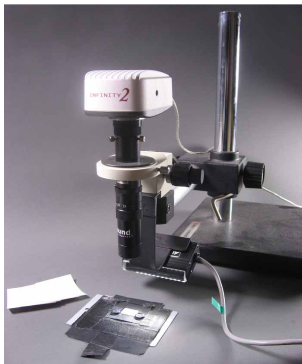
FIG. 1. System for raking-light close-up image acquisition.
