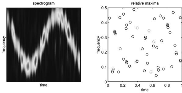
Figure 1: Example of a monocomponent frequency modulated signal, at 5dB SNR. Left : spectrogram; Right : (2D) distribution of the relative maxima
