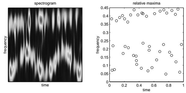
Figure 3: Example of a two-component frequency modulated signal, at 5dB SNR. Left : spectrogram; Right : (2D) distribution of the relative maxima
