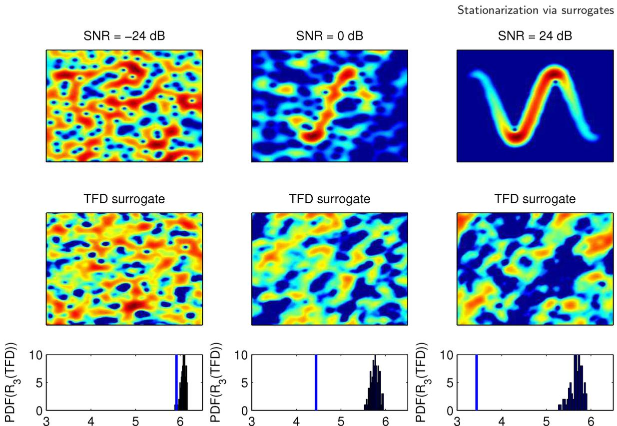
**Figure 5.** *Transient detection.* The detection test is applied to a chirp embedded in a white Gaussian noise with several SNR (−24, 0 and 24 dB). From top to bottom: TFD of the signal with noise, TFD surrogate with positivity constraint; statistics for the test (Rényi entropy of order 3): (blue) vertical bar for the signal, (black) histogram for the surrogates.
