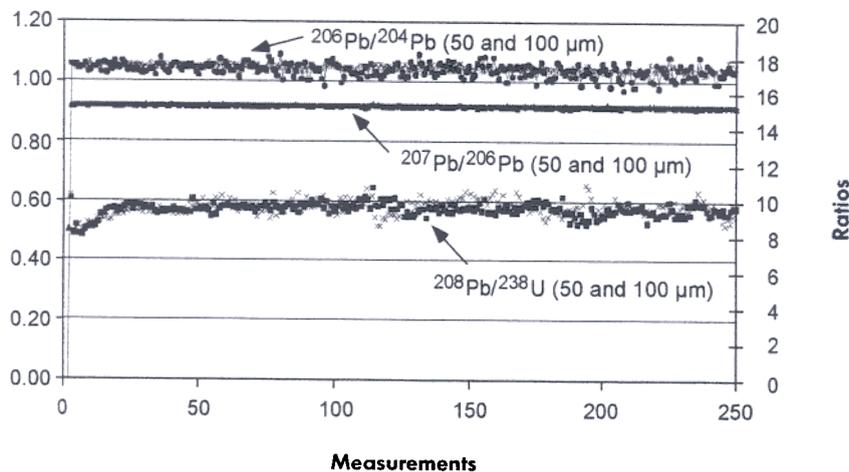
**Figure 5. NIST SRM 610 measurements for 50 and 100  $\mu\text{m}$  craters with the Plasma 54 ICP-MS. Each symbol represents 2 seconds. The total acquisition time was 8 minutes.**
