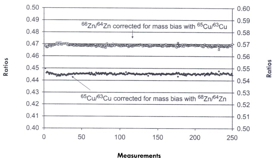
**Figure 6.** Cu and Zn measurements, made with the Plasma 54 ICP-MS, on a brass nut sample.
