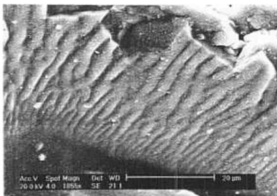
**Figure 2. SEM photograph showing cracks on NIST SRM 610 glass reference material.**
