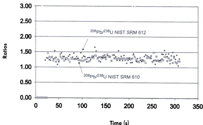
**Figure 3.** <sup>208</sup>Pb/<sup>238</sup>U ratios measured with the 157 nm laser and VG PQ2+ ICP-MS. Ratios for NIST SRM 610 were corrected to the same Pb/U ratio as NIST SRM 612.
