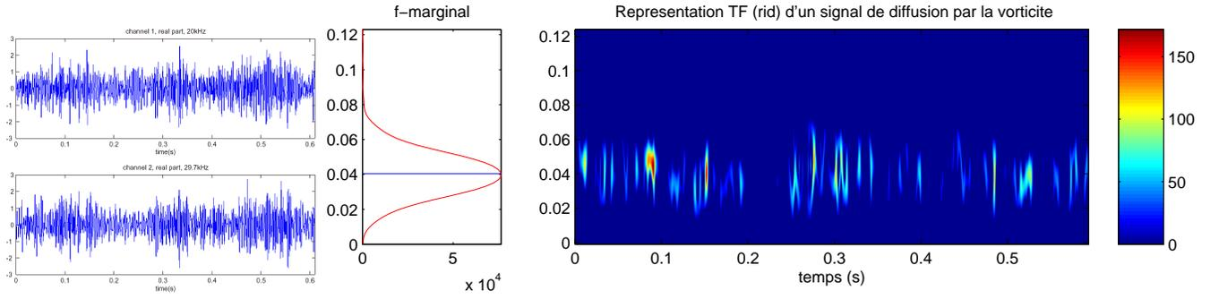
Figure 4: Measurement of vorticity by acoustic scattering [BMW99]. Left: examples of recorded signals for two different scattered waves at the same time by the same volume: they both represent the same  $\tilde{\omega}_i(\mathbf{k}, t)$  along time  $t$ . Right: quadratic time-frequency representation of one signal, exhibiting packets of structured vorticity advected through the measurement volume. [BMW99]
