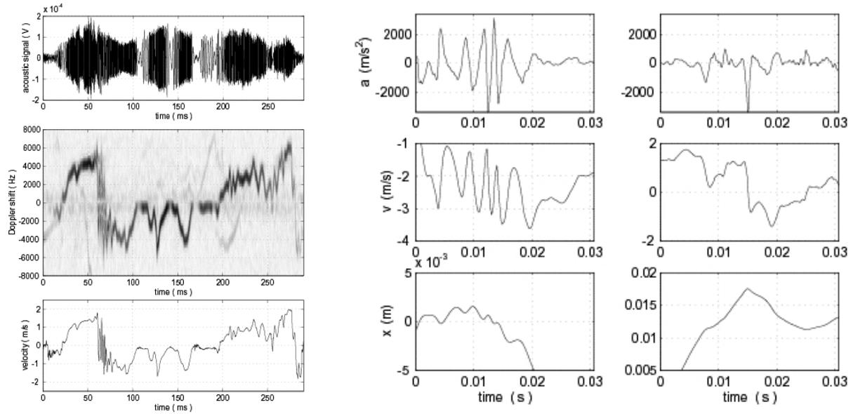
Figure 3: Lagrangian velocity of a particle in turbulence (from [MMMP01]). Left: the Doppler signal whose instantaneous frequency gives the velocity of the tracked solid particle in a turbulent fluid, and its time-frequency representation. Right: acceleration, velocity and trajectory, reconstructed for two components from the measurement of velocity by Doppler effect.
