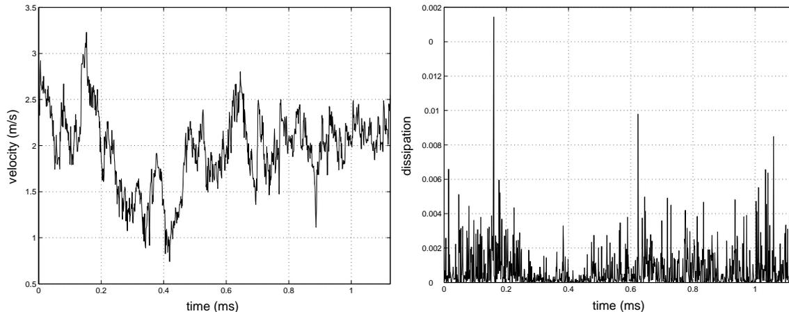
Figure 1: Left: a typical Eulerian velocity signal  $v(t)$ . Right: its corresponding dissipation (derivative of the squared velocity). Those signals were measured by Pietropinto *et al.* as part of the GReC experiment [PPB<sup>+</sup>03] of fluid turbulence in low temperature gaseous helium.
