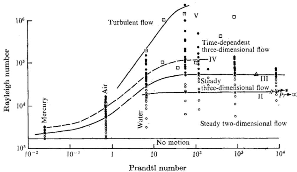
FIGURE 4. Regime diagram. ○, steady flows; ●, time-dependent flows; ★, transition points with observed change in slope; □, Rossby's observations of time-dependent flow; □, Willis & Deardorff's (1967*a*) observations for turbulent flow; △, Silveston's point of transition for time-dependent flow (see text).
