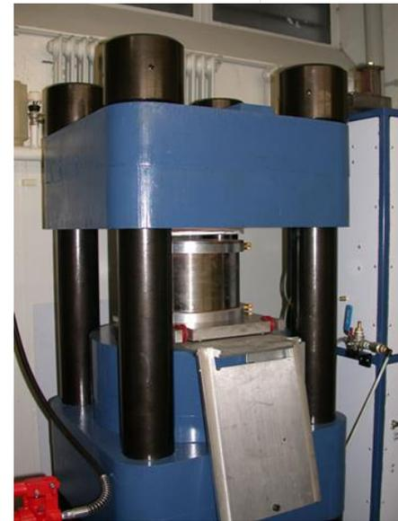
Piston cylinder apparatus
