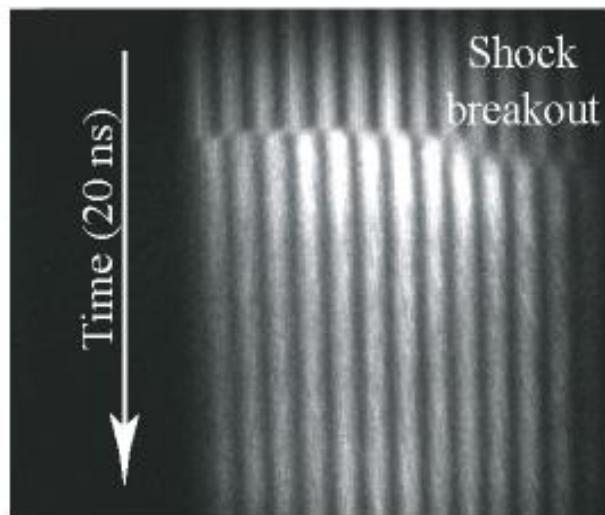
Image of interferometry of the rear face (VISAR)
