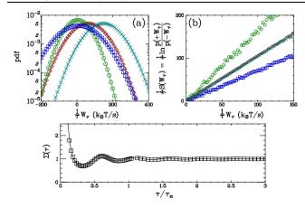
FIG. 3 (color online). SSFT with a ramp forcing. (a) PDF of  $W_{\tau}$  for various  $\tau/\tau_{\alpha}$ : 0.019 ( $\bigcirc$ ), 0.31 ( $\Box$ ), 2.09 ( $\diamondsuit$ ), and 4.97 ( $\times$ ). (b) Corresponding functions  $S(W_{\tau})$ . (c) The slope  $\Sigma(\tau)$  of  $S(W_{\tau})$  is plotted versus  $\tau$  [ $\Box$ : experimental values; continuous line: theoretical prediction Eq. (10) with no adjustable parameter].
