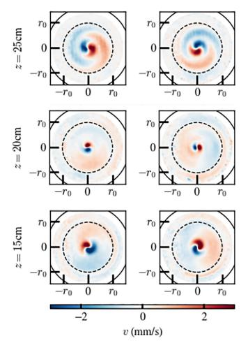
FIG. 9. Horizontal views with a laser sheet at height  $z=25\,\mathrm{cm}$ ,  $20\,\mathrm{cm}$ , and  $15\,\mathrm{cm}$  from top to bottom, showing  $v_r$  (left) and  $v_\varphi$  (right). In this experiment N=0,  $f_c=-1.05\,\mathrm{rads}^{-1}$  (experiment B in Table I) and  $\omega_0/f_c=0.767$ . The velocity field is filtered around the forcing frequency with a window  $0.05f_c$  wide.
