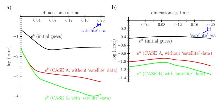
**Fig. 11.** Dynamical evolution of  $L_2$  errors (logarithmic value) for the magnetic field (a) and the fluid velocity (b). Black lines: errors for initial guesses. Green (red) lines: errors for assimilation results that do (not) incorporate the data obtained by a dense virtual network of magnetic stations, which aims at mimicking the satellite era – the blue segment on each panel –, spanning the last 5% of model integration time.
