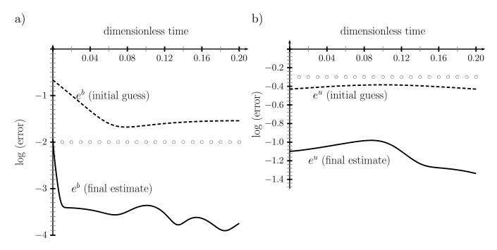
Fig. 5. Dynamical evolution of  $L_2$  errors (logarithmic value) for the magnetic field (a) and the fluid velocity (b). Dashed lines: errors for initial guesses. Solid lines: errors after variational assimilation. Circles represent instants are which magnetic observations are made. In this particular case, nt=20 and  $n^{S}=20$ .
