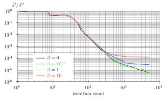
**Fig. 10.** Convergence behaviour for different constraint levels  $\beta$ . The ratio of the current value of the misfit  $J^l$  (normalized by its initial value  $J^0$ ) is plotted against the iteration count *l*.  $\beta$  measures the strength of the constraint imposed on the state relative to the observations.
