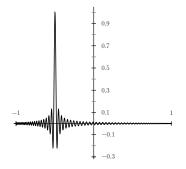
**Fig. 1.** An example of a basis function used to discretize the MHD model in space. This particular Lagrangian interpolant,  $h_{50}^{150}$ , is obtained for a polynomial order N=150, and it is attached to the 51st Gauss–Lobatto–Legendre point.
