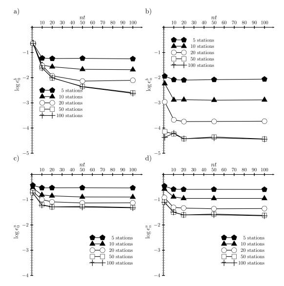
Fig. 6. Systematic study of the response of the one-dimensional MHD system to variational assimilation. Shown are the logarithms of  $L_2$  errors for the t=0 (a) and t=T (b) magnetic field, and the t=0 (c) and t=T (d) velocity field, versus the number of times observations are made over [0,T], nt, using spatial networks of varying density ( $n^{S}=5$ , 10, 20, 50 and 100).
