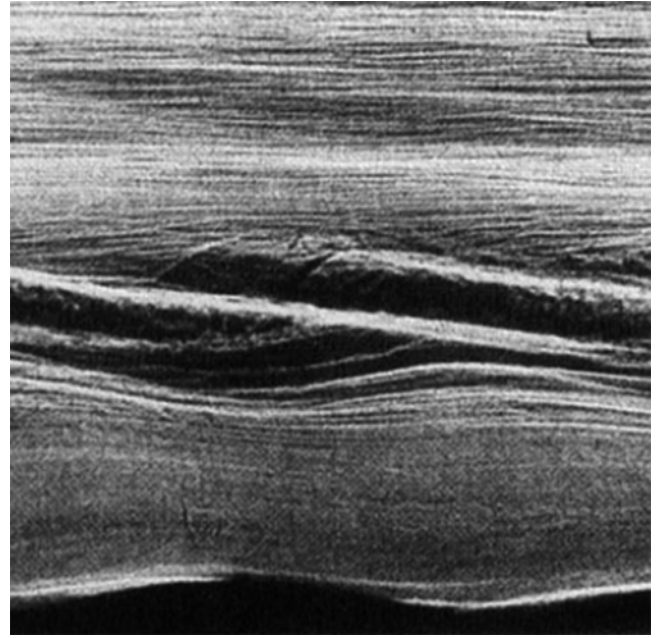
Figure 10.1. Internal wave breaking near a critical layer as visualized by shadowgraph. Reprinted from Figure 7 of Koop and McGee [1986].
