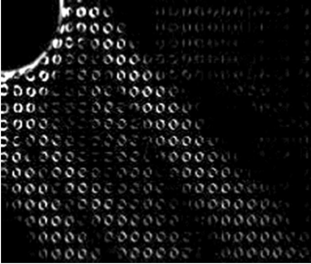
Figure 10.4. Pattern of internal waves generated by an oscillating cylinder in the upper left-hand corner as visualized by qualitative synthetic schlieren applied to a pattern of equally spaced dots behind the tank. Adapted from Figure 7c of Dalziel et al. [2000].
