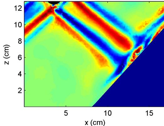
Figure 2: Horizontal density gradients visualized by synthetic Schlieren in critical conditions  $\theta = \alpha = 48^\circ$ . The excitation frequency is  $f = 0.3$  Hz.
