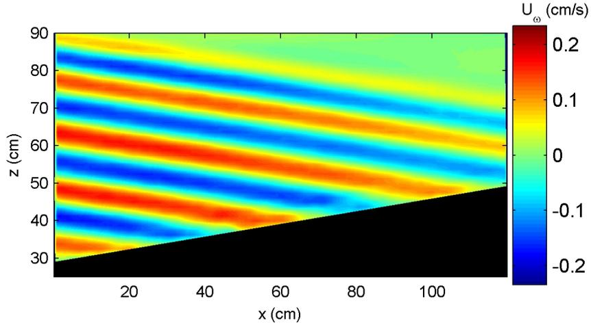
Figure 5: Horizontal velocity field filtered at the fundamental frequency for  $\theta = 8^\circ$  and  $\alpha = 9.5^\circ$ .
