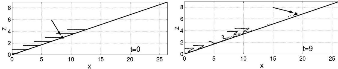
Figure 6: Passive tracers initially located on iso-density lines and advected by the velocity evaluated for critical incidence.
