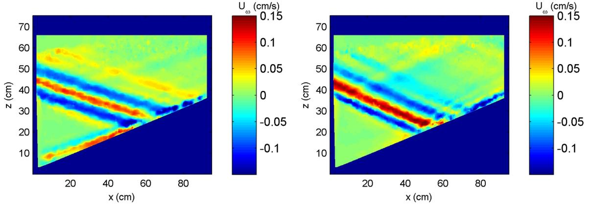
Figure 3: Horizontal velocity field, filtered at the excitation frequency when  $\theta - \alpha = -3^\circ$  (left panel) and  $1.8^\circ$  (right panel).
