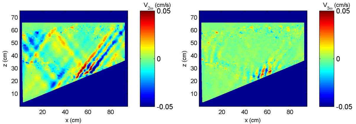
Figure 4: Vertical velocity field filtered at the second harmonic (left panel) and third harmonic (right panel) in a super-critical case ( $\theta - \alpha = 1.8^\circ$ ).
