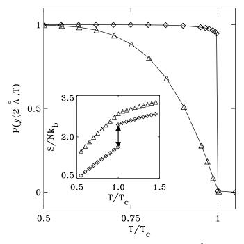
FIG. 4. The fraction of bound base pairs P(y < 2 Å, T) as a function of the  $T/T_c$  for the type I (triangles) and II (diamonds). Inset: the entropy  $S(T)/Nk_B$  (symbols as in main figure); the length of the double arrow represents the estimate of the melting entropy obtained from the scaling Eq. (6). The solid lines are "guides to the eye."
