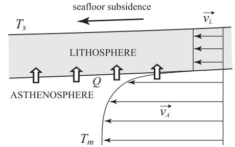
**Fig. 2.** Sketch of the lithosphere-asthenosphere interaction. In our model, the velocity in the asthenosphere is faster than the overlying plate and almost constant over the asthenosphere depth, except for a thin upper boundary layer.  $T_s$  and  $T_m$  indicate the seawater and mantle temperature, respectively. The heat flux  $Q$  at the base of the lithosphere is imposed by the flow within the asthenosphere.
