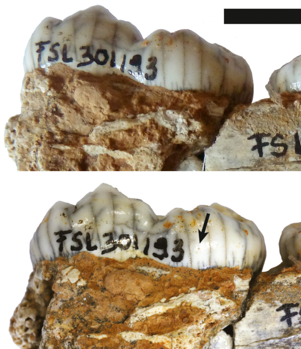
FIG. 3. Ursus arctos molar from Jaurens, France sampled in this study. The top picture is before sampling. The arrow in the bottom picture shows the microdrill perforation after sampling highlighting that a minimal amount of sample is needed for calcium isotope measurements. Scale bar represents 1 cm.
