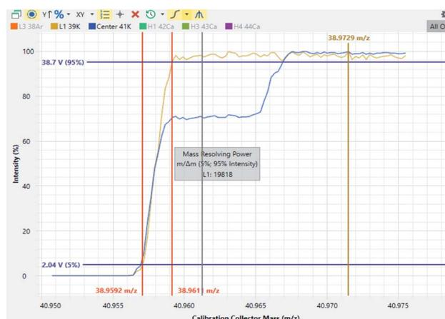
**Fig. 1** Peak scan of the SRM-3141a solution at  $1\ mg\ L^{-1}$  using the set of parameters given in Table 2 showing the peak shape of the  $m/z$  value 39 (yellow) with the automated calculation of the resolution (5, 95% of  $m/z$  value 39) on the ascending edge of the peak. Potassium isotope ratio measurement was performed at the middle of the  $^{40}ArH^+$  interference-free plateau of the  $^{41}K^+$  peak. The software used is an adapted version of Qtegra for MC-ICP-MS analysis.
