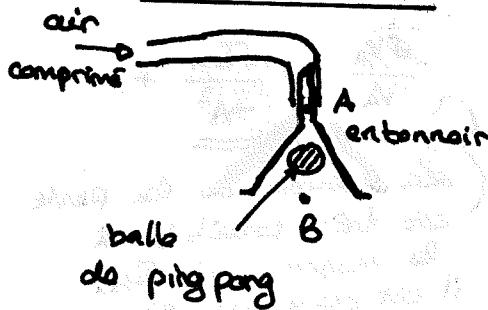
$$\left\{ \begin{array}{l} \text{Conservation du débit: } V_A S_A = V_B S_B \\ \text{R. de B: } P_B + \frac{1}{2} \rho V_B^2 = P_A + \frac{1}{2} \rho V_A^2 \end{array} \right. \Rightarrow S_A < S_B \Leftrightarrow V_A > V_B \Rightarrow P_A < P_B$$
