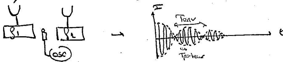
$$I = 2 I_0 \cos\left(\frac{\omega_1 - \omega_2}{2} t\right) \cos\left(\frac{\omega_1 + \omega_2}{2} t\right)$$
