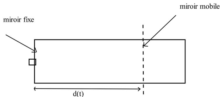
FIGURE 2 – Cavit  r sonante de Fabry P rot
