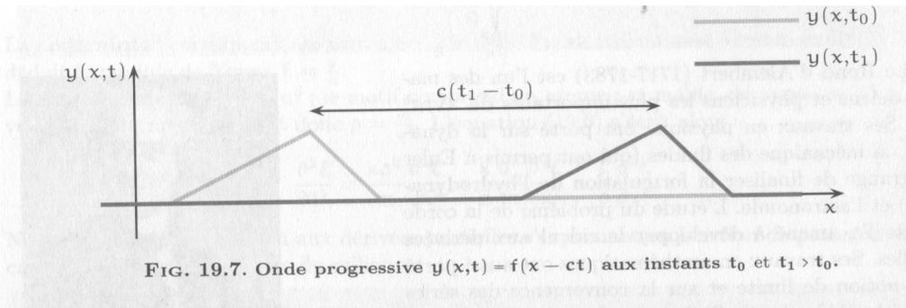
FIG. 19.7. Onde progressive  $y(x, t) = f(x - ct)$  aux instants  $t_0$  et  $t_1 > t_0$ .
