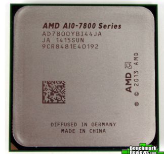
AMD 5th (Kaveri) CPU-GPU chip (quad-core, 512 Radeon cores)
