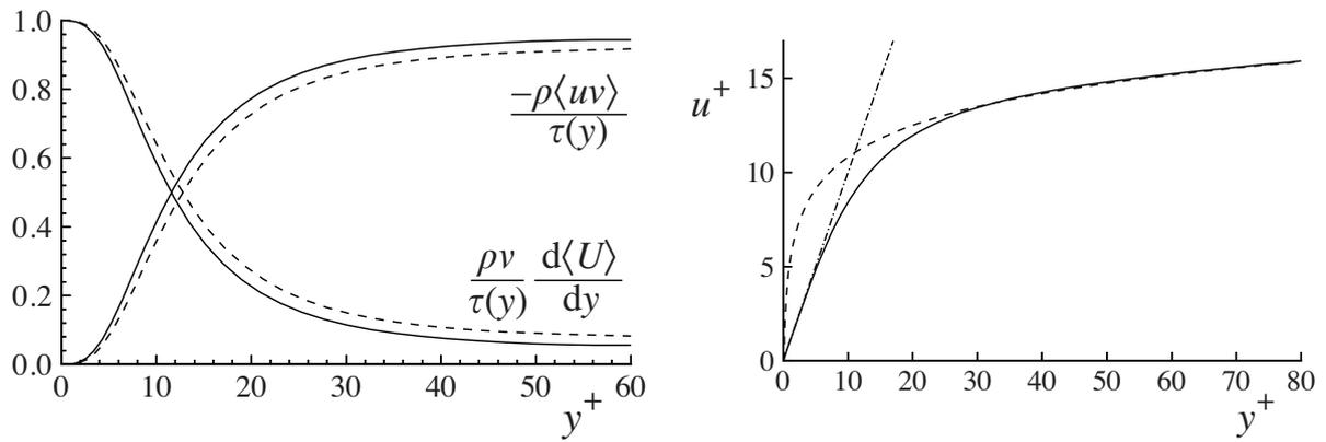
Figure 1: Relative contributions of the viscous and Reynolds stresses (left) and mean axial velocity (right) as a function of the distance to the wall, obtained in Direct Numerical Simulations of a channel flow at  $Re = 13750$ .
