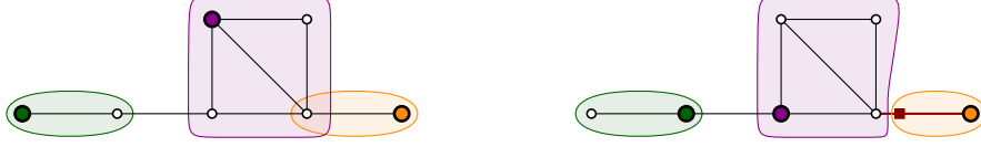
Figure 6: A similar transformation for arbitrary graphs does not work. On the right side we have the transformed instance with a feasible solution that does not correspond to a solution in the original setting.
