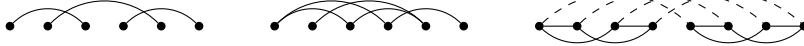
FIGURE 7. A strict queue; a queue; and a 2-queue-layout of the cube, partitioned in solid and dashed edges.
