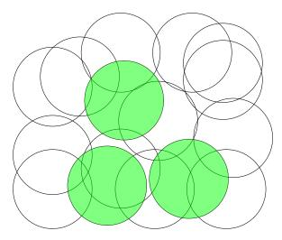
Frequency assignment in broadcast networks k-COLORING is NP-hard for any integer  $k \ge 3$  the problem can be 3-approximated
