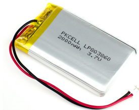
(c) 2000 mAh LiPoly battery.
