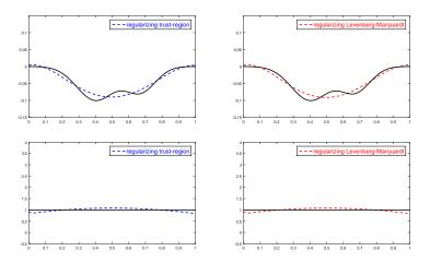
Left: regularizing TR, Right: regularizing LM , Solid line: solution of the original problem.
