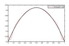
Computed solution,  $x_0 = 1e$ ,  $\delta = 1.e - 2$ . **Left**: trapezoidal rule, **Right**: rectangular rule, **Solid** line: solution of the original problem.
