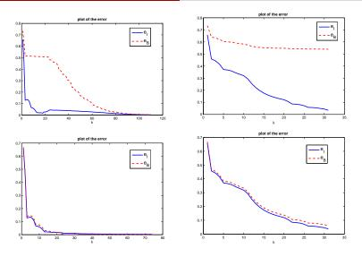
$e_l$  = error computed on the points inside the interval,  $e_B$  = border error. **Upper part**: trapezoidal rule, left:  $\delta = 0$ , right:  $\delta = 1.e - 2$ . Lower part: rectangular rule, left:  $\delta = 0$ , right:
