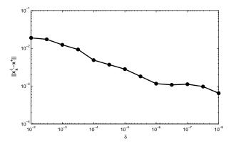
Logarithmic plot of the error  $||x_{k^*(\delta)}^{\delta} - x^{\dagger}||$  as a function of the noise level  $\delta$ .
