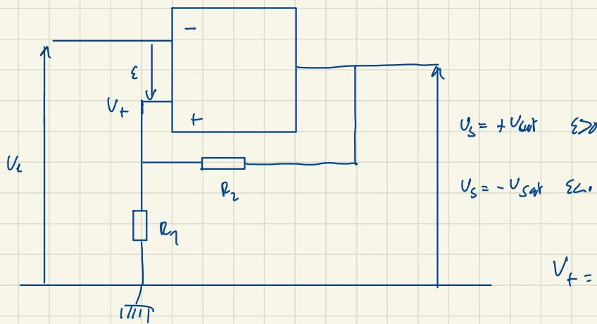
$$U_f = U_S \cdot \frac{R_L}{R_1 + R_L}$$
