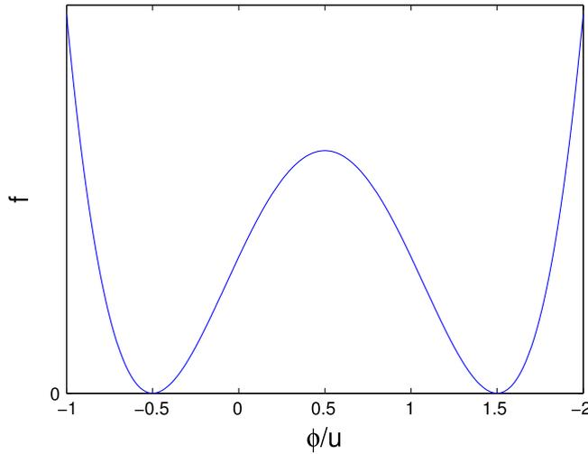
**Fig. 7.** The double well shape of the specific free energy  $f(\phi)$  (see Eq. (80)). The function  $f(\phi)$  is even and possesses two minima at  $\phi = \pm u$ . At equilibrium, at zeroth order in  $R$ , the physical system will be described by two phases corresponding to each of these minima.
