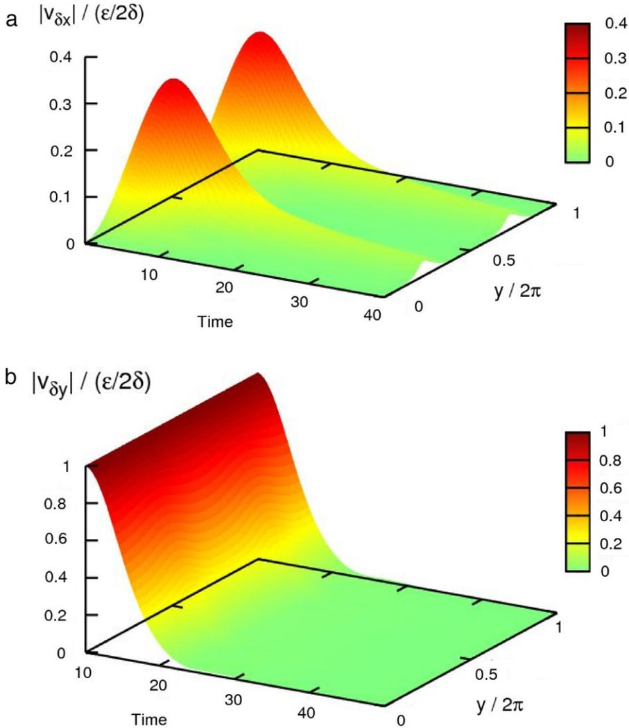
**Fig. 31.** The space-time series of perturbation velocity components,  $|v_{\delta,x}(y, t)|$  (a) and  $|v_{\delta,y}(y, t)|$  (b), for the initial perturbation profile  $\cos(x/\delta)$  in a doubly periodic domain with aspect ratio  $\delta = 1.1$ . Both the components relax towards zero, showing the asymptotic stability of the Euler equations.
