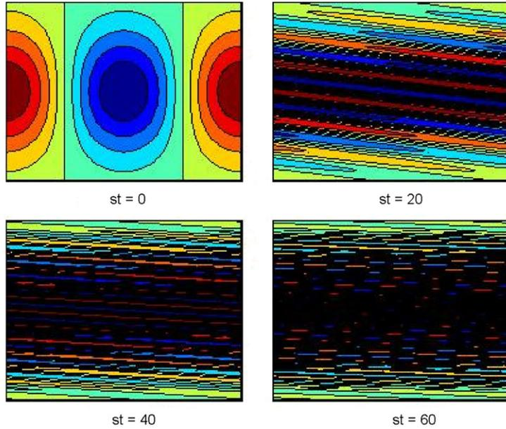
**Fig. 29.** Evolution of  $\omega(x, y, t)$  from an initial vorticity perturbation  $\omega(x, y, 0) = \omega_1(y, 0) \cos(x)$ , by the linearized 2D Euler equations close to a shear flow  $U(y) = \sigma y$ .
