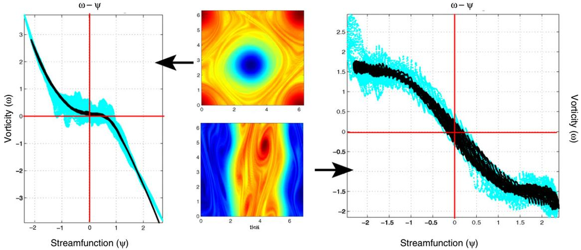
**Fig. 23.**  $\omega$ - $\psi$  scatter-plots (cyan). In black the same after time averaging (averaging windows  $1 \ll \tau \ll 1/\nu$ , the drift due to translational invariance has been removed). Left: dipole case with  $\delta = 1.03$ . Right: unidirectional case  $\delta = 1.10$ .
