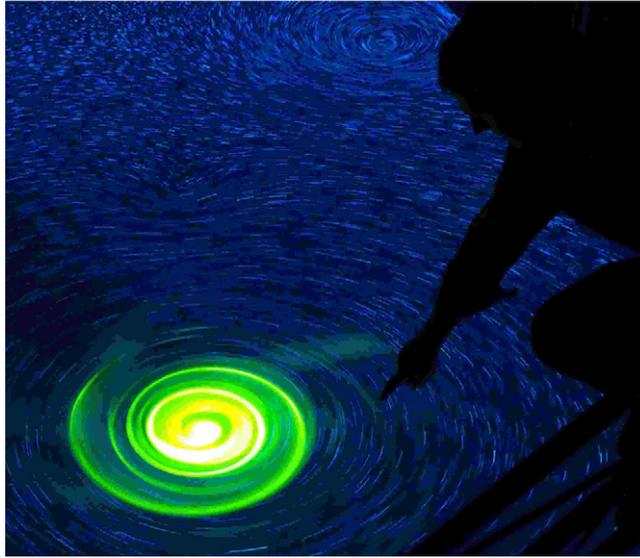
**Fig. 2.** Experimental observation of a 2D long lived coherent vortex on the 14 m diameter Coriolis turntable (photo gamma production).
