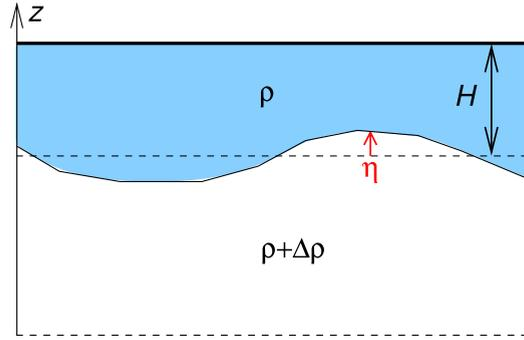
**Fig. 3.** Vertical structure of the 1.5-layer quasi-geostrophic model: a deep layer of density  $\rho + \Delta\rho$  and a lighter upper layer of thickness  $H$  and density  $\rho$ . Because of the inertia of the lower layer, the dynamics is limited to the upper layer.
