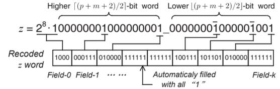
Fig. 2. The proposed recoding scheme for variable  $z$ .
