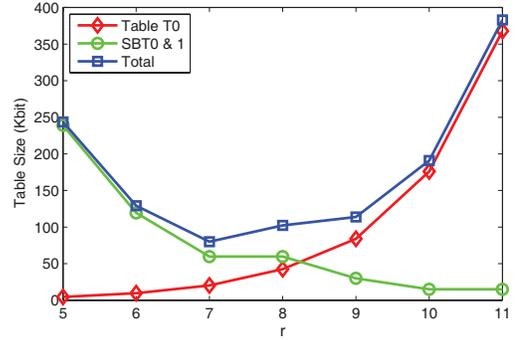
Fig. 4. The estimated lookup table sizes for different values of  $r$  when  $n = 24, p = 24$ . For  $r = 11$ , the total lookup size is 384 Kbits, which is 4.5 times larger than the lookup size for  $r = 7$  (85.7 Kbits).
