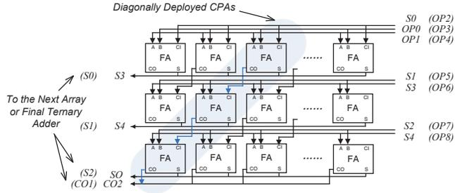
Fig. 3. The proposed parallel linear array structure for a [9:3] compressor. The output signals  $SO$ ,  $CO1$  and  $CO2$  are fed to a ternary adder, which can support 3-input addition ( $A+B+C=D$ ) with the same amount of resource overhead and similar speed as a simple 2-input adder. FA: full-adder.
